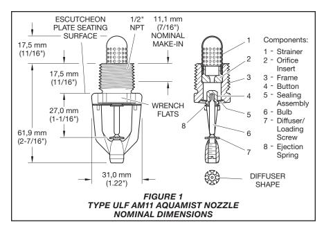
**Note:** Do not attempt to compensate for insufficient adjustment in the escutcheon plate by under or overtightening the nozzle. Re-adjust the position of the nozzle fitting to suit.
